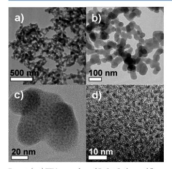
**Figure 1.** (a–c) TEM images of ground Fe<sub>x</sub>O<sub>y</sub>@C spheres at different magnifications, showing cross-linked nanorods inside. (d) HRTEM image of one carbonaceous nanorod embedded with iron oxide nanoparticles. Reproduced with permission from ref 61. Copyright 2010 American Chemical Society.<sup>61</sup>
