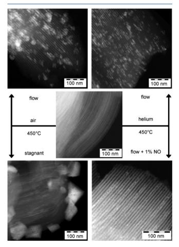
**Figure 4.** HAADF-STEM images of  $Ni_3(NO_3)_2(OH)_4/SBA-15$  obtained after drying at 120 °C (center) and of NiO/SBA-15 obtained after different thermal treatments at 450 °C, as indicated. Reproduced with permission from ref 112. Copyright 2007 John Wiley and Sons.<sup>112</sup>
