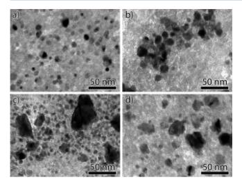
**Figure 10.** TEM of microtomed 50 nm slices of catalyst particles after 50 h on-stream. (a) Ni-D8, (b) Ni-C9, (c) Ni-C4, and (d) Ni-C3 (C = closer, D = dispersed, the number refers to grain size/nm of Ni NPs before reaction). Reproduced with permission from ref 94. Copyright 2014 John Wiley and Sons.<sup>94</sup>
