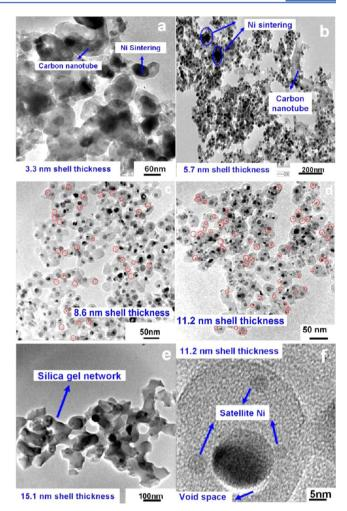
**Figure 8.** TEM images of spent catalysts with different shell thicknesses after 20 h of reaction: (a-e) low magnification and (f) high magnification for Ni-yolk@Ni@SiO<sub>2</sub> with 11.2 nm shell thickness. Reproduced with permission from ref 52. Copyright 2014 American Chemical Society.<sup>52</sup>
