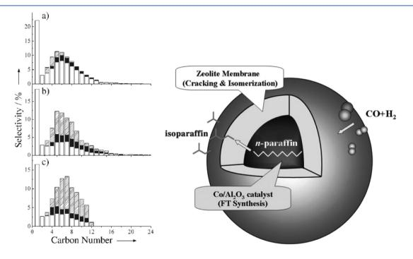
**Figure 13.** Left are the product distributions for (a) conventional Co/Al<sub>2</sub>O<sub>3</sub>, (b) the physical mixture of Co/Al<sub>2</sub>O<sub>3</sub> and beta-zeolite, and (c) the zeolite-coated Co/Al<sub>2</sub>O<sub>3</sub> catalyst.  $\Box$  = *n*-paraffin,  $\blacksquare$  = olefin, hatched = isoparaffin. The right is the model of the core@shell catalyst. Reproduced with permission from ref 32. Copyright 2008 John Wiley and Sons.<sup>32</sup>
