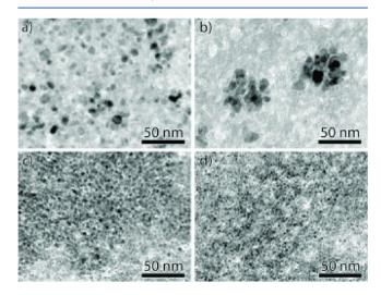
**Figure 9.** Bright-field TEM of 50 nm thick slices of Ni/SiO<sub>2</sub> catalysts after reduction: (a) Ni-D8, (b) Ni-C9, (c) Ni-C4, and (d) Ni-C3 (C = closer, D = dispersed, the number refers to grain size/nm of Ni NPs before reaction). Reproduced with permission from ref 94. Copyright 2014 John Wiley and Sons.<sup>94</sup>
