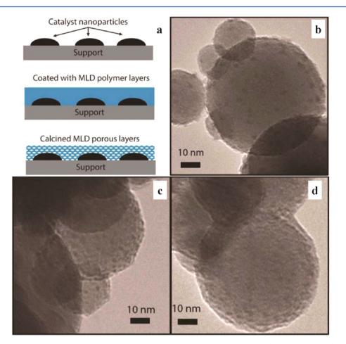
Figure 7. (a) Schematic representation of MLD coating process to produce porous alumina overlayers. (b) Ni nanoparticles (2-5 nm dark particles) deposited on spherical alumina; Ni/Al<sub>2</sub>O<sub>3</sub> nanoparticles coated by (c) 5-MLD cycles and (d) 10-MLD cycles. The hybrid polymer–inorganic MLD layer is the lighter layer encircling the spheres in c and d. Reproduced with permission from ref 164. Copyright 2014 American Chemical Society.<sup>164</sup>
