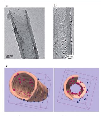
**Figure 2.** (a) Typical 2D-TEM images of the sample "metal inside", used to reconstruct its volume. (b) Longitudinal section through the reconstructed volume. (c) Modeling of the reconstructed volume: (pink) carbon nanotubes, (red) Ni NPs inside the tube, (blue) Ni NPs on the external surface. Adapted with permission from ref 91. Copyright 2009 American Chemical Society.<sup>91</sup>
