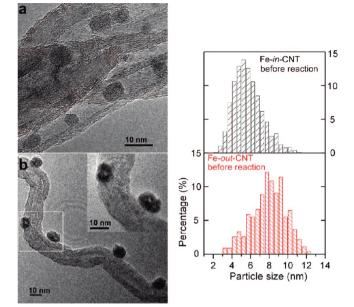
**Figure 11.** TEM images and particle size distribution of activated catalysts (a) Fe-*in*-CNT and (b) Fe-*out*-CNT before reaction. Reproduced with permission from ref 76. Copyright 2008 American Chemical Society.<sup>76</sup>
