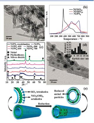
**Figure 3.** (a) TEM image of the as-prepared Ni/PS<sub>n</sub>. (b) TPR profiles of Ni/SiO<sub>2</sub> catalysts. (c) X-ray diffraction (XRD) patterns of Ni/PS<sub>n</sub> before and after calcination and upon reduction at different temperatures. (d) TEM image of Ni/PS<sub>n</sub>-600. (e) Schematic model of Ni/PS<sub>n</sub> and Ni/PS<sub>n</sub> after reduction. Reproduced with permission from ref 92. Copyright 2013 The Royal Society of Chemistry.<sup>92</sup>
